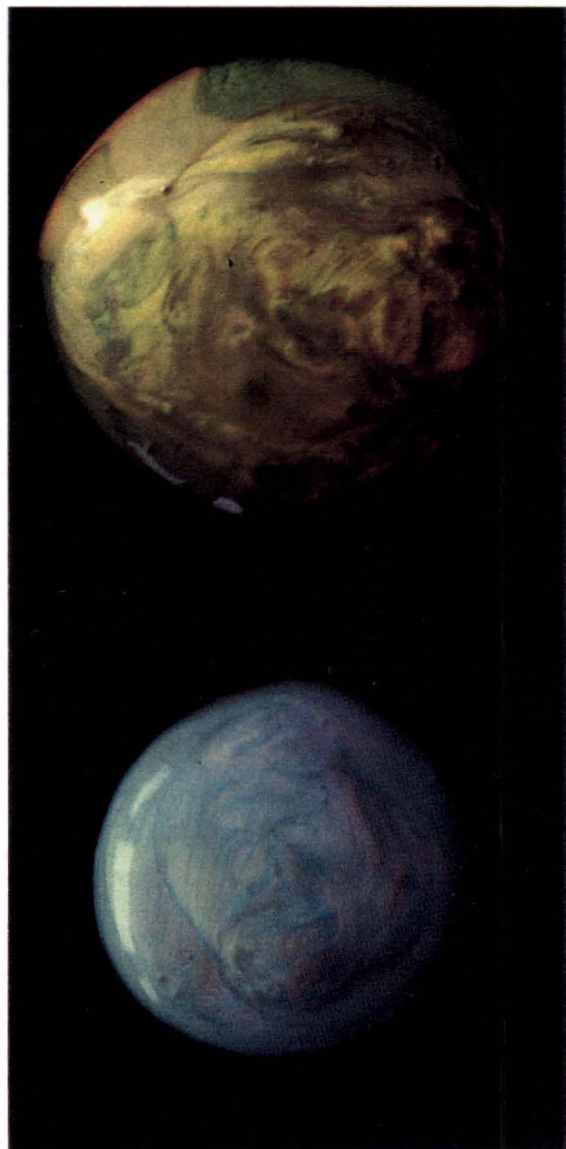
Figs 1 & 2: "Pym water" — droplets of a cholesteric liquid crystal showing reflection colour and distinct veins.
